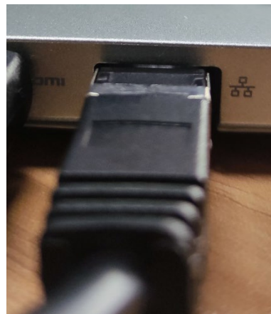
Figure 6 Computer Ethernet port 1
